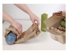
The PadPak LC is the fastest paper cushioning solution on the market. The high output allows a maximum box throughput. The converter forms single layer paper into pads which can be used to protect products during shipment. The individual bundles of paper, with gluing strip, ensure the converter is easy to load and runs at high speed. The paper pad can be used for cushioning, blocking and bracing or wrapping.
